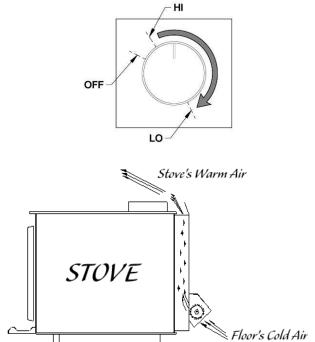
CAUTION: ENSURE THAT THE BLOWER'S POWER CORD IS NOT IN CONTACT WITH ANY SURFACE OF THE STOVE TO PREVENT ELECTRICAL SHOCK OR FIRE DAMAGE. DO NOT RUN THE POWER CORD BENEATH THE STOVE.
